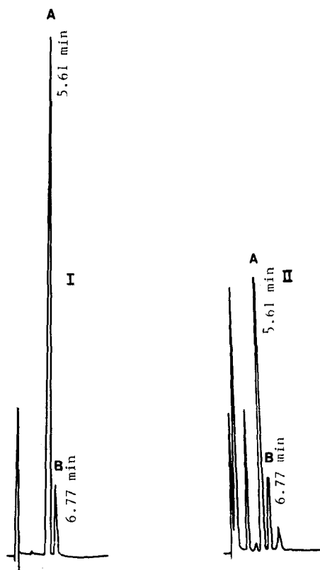
Figure 2 I. Chromatograms of cefazolin (A), and 7-hydroxycoumarin (B) in peritoneal dialysis solution.
